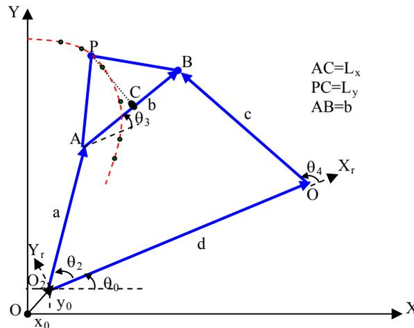
Figure 1: Four-bar mechanism in global coordinate frame
