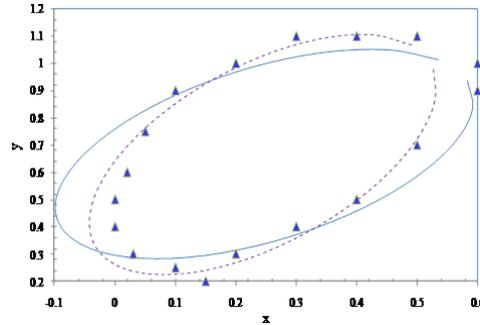
Figure 4: Coupler curve for case 2 (solid: HSO, dotted: GA-DE [7],  $\Delta$ : Desired)
