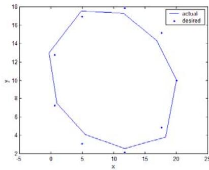
Figure 2: Coupler curve for case-1
