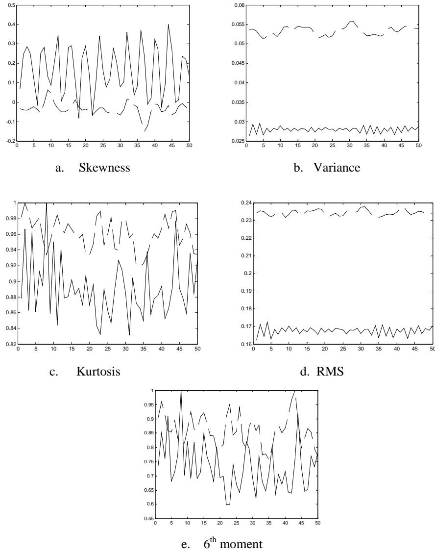
Figure 1: Variation of parameters for normal (dotted line) & faulty (solid line) data sets.
