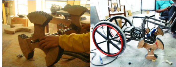
Fig 9 i) central shaft with Y shaped wooden wheel, ii) modified wheelchair chassis
