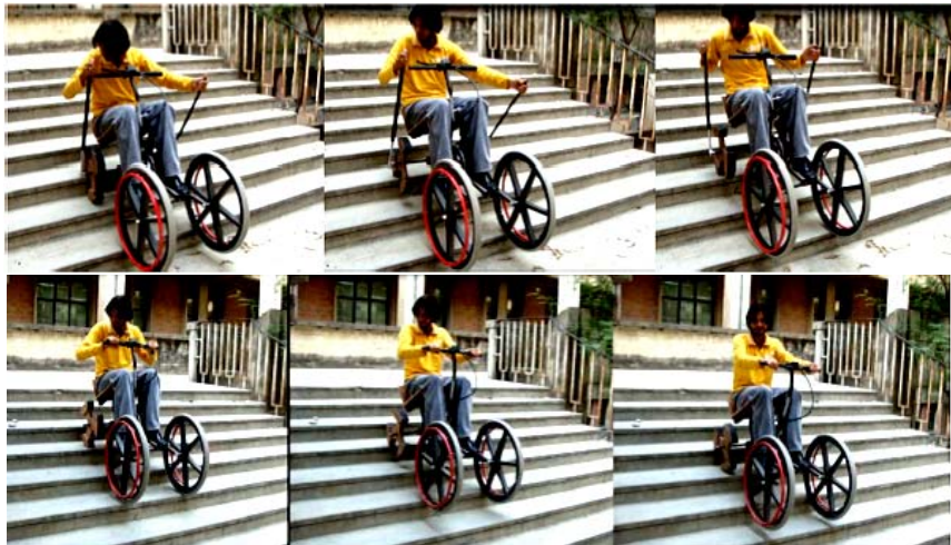
Fig 10 Prototype climbs up with lever ratchet arrangement and climbs down with disk brake arrangement respectively
